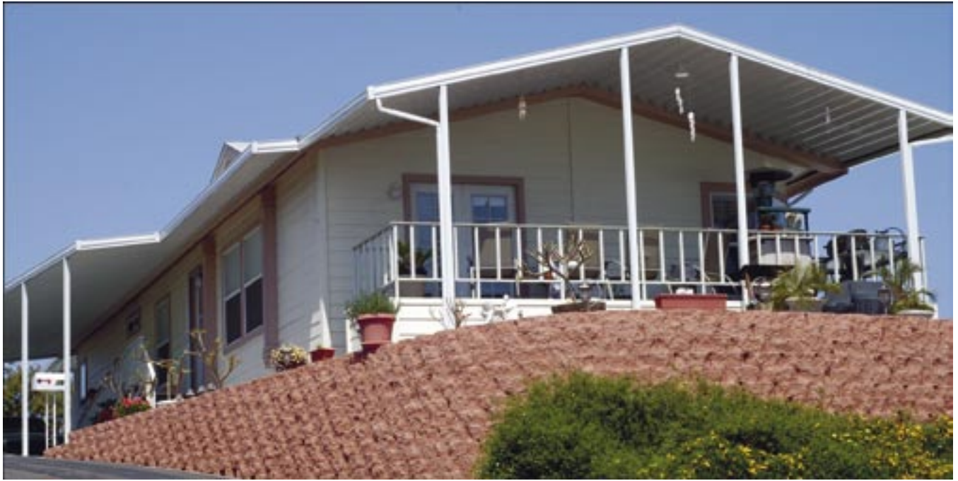
One of many HUD-Code homes that Viva Homes has placed in the Rancho Jamacha park in Spring Valley, CA. They are characterized by decorative block retaining walls to secure extra space and are often double-section units.
